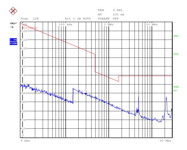
Resolution bandwidth: 200 Hz for 9 kHz  $\leq$  f  $\leq$  150 kHz 9 kHz for 150 kHz  $\leq$  f  $\leq$  30 MHz
