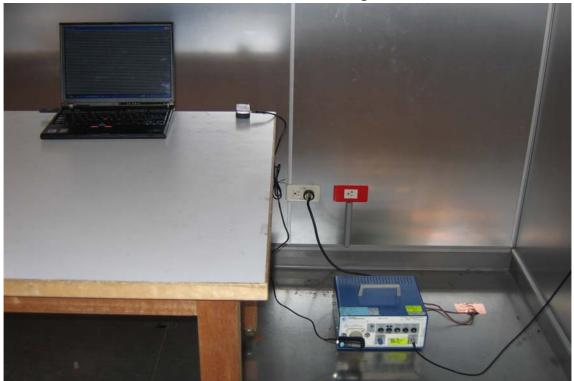
**Conducted Emission Set up Photo**
