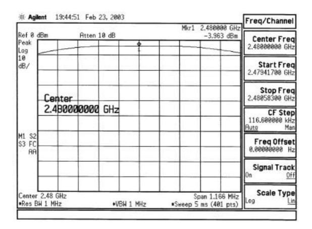
At the 2480 Mhz , The measured output power is -3.963 dBm.
