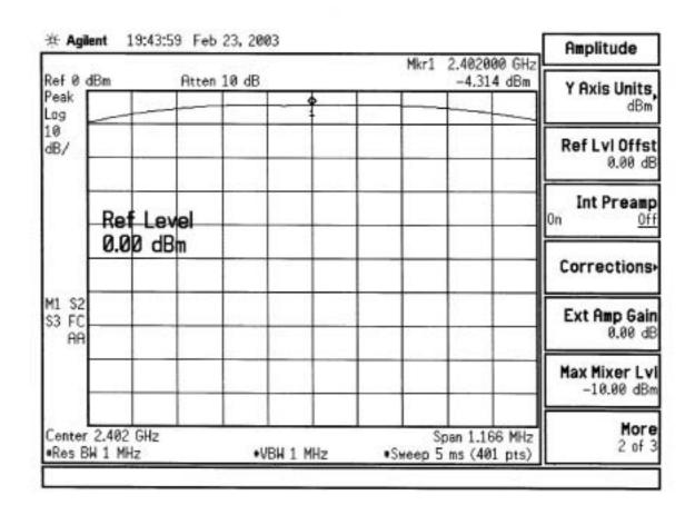
At the 2402Mhz , The output power is -4.314 dbm.
