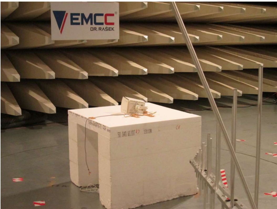
Photo A1-2: Radiated emissions measurement at 3 m distance, 30 MHz – 1000 MHz
