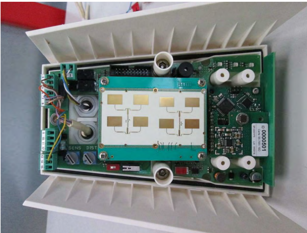
Photo A3-6: Assembled PCBs
