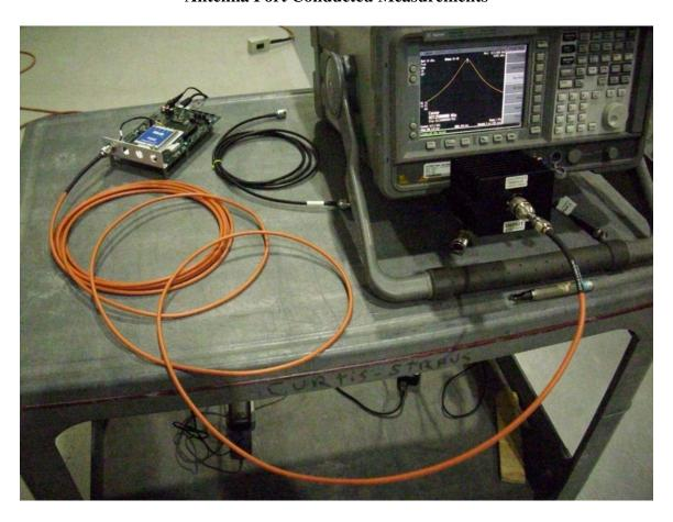
**Antenna Port Conducted Measurements**
