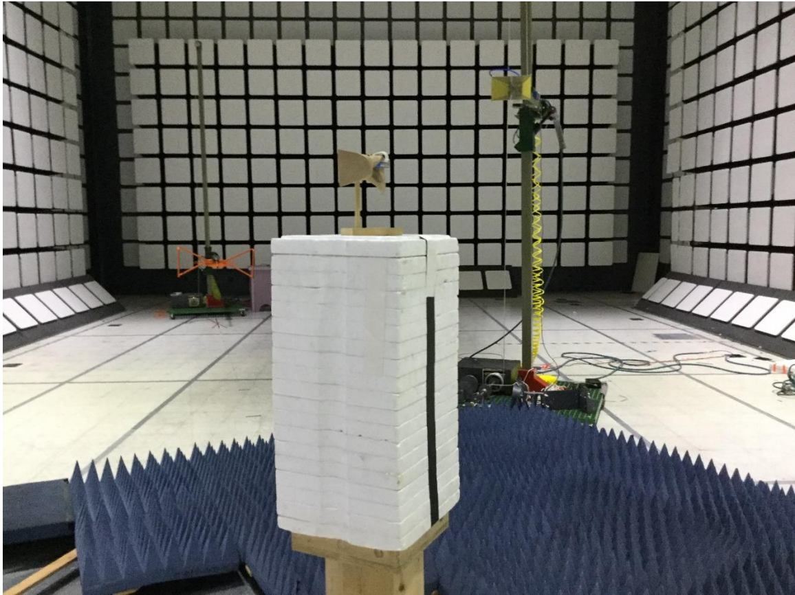
Figure 2 - Radiated Emissions Test Setup, Vertical, 1GHz – 25GHz
