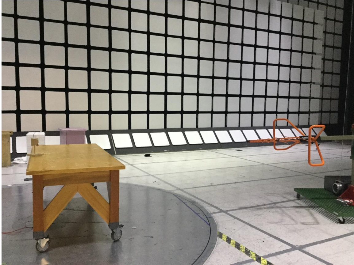
Figure 45 – Radiated Emissions Test Setup, 30MHz – 1GHz
