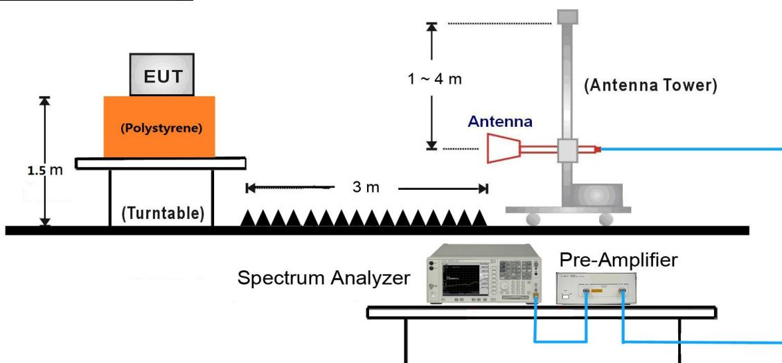
18GHz ~25GHz Test Setup:
