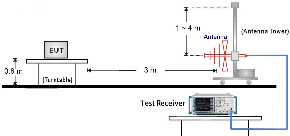
1GHz ~ 18GHz Test Setup:
