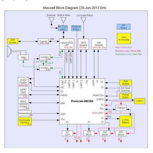
The processor is the central element of the 9560 system and is running a Linux operating system with adequate performance requirements for a SIP server and other web services via WIFI.
