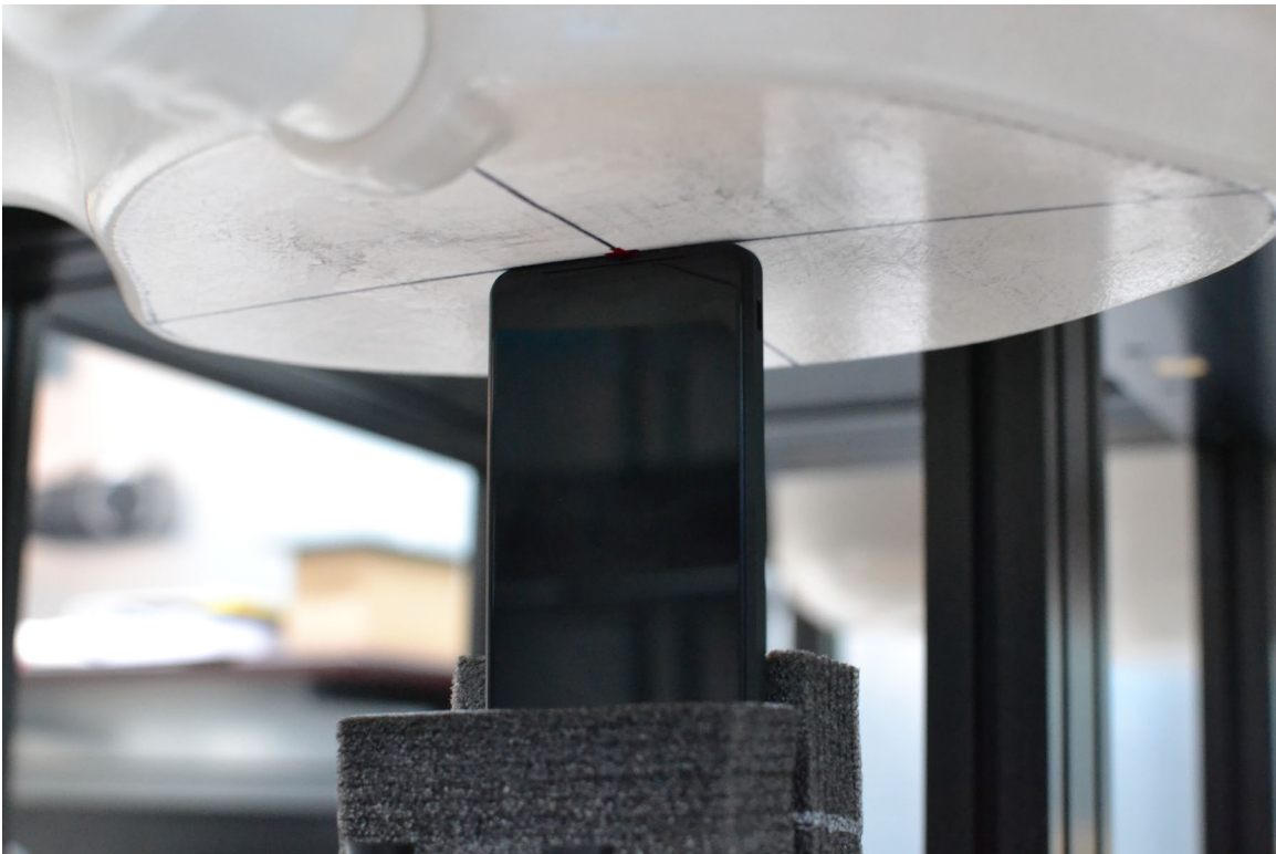
SAR Test Setup Photo 12 – Phablet, Bottom Edge, 0 mm
