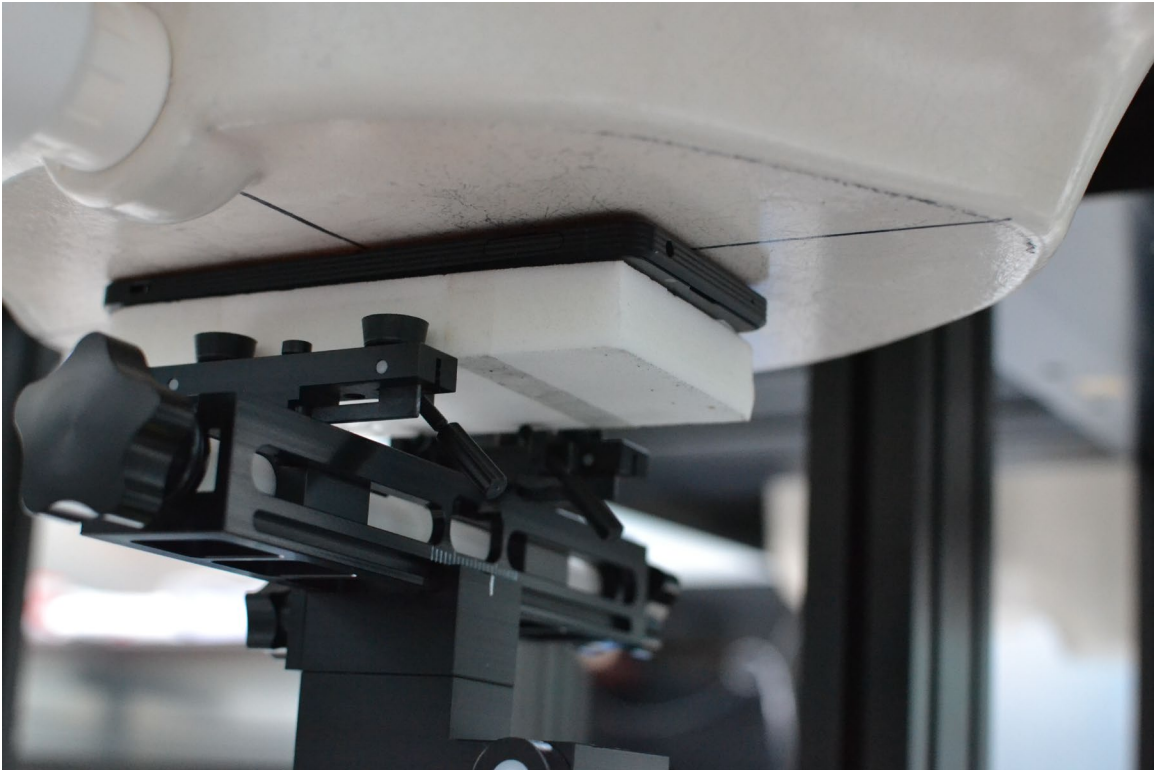
SAR Test Setup Photo 6 – Phablet, Back Side, 0 mm
