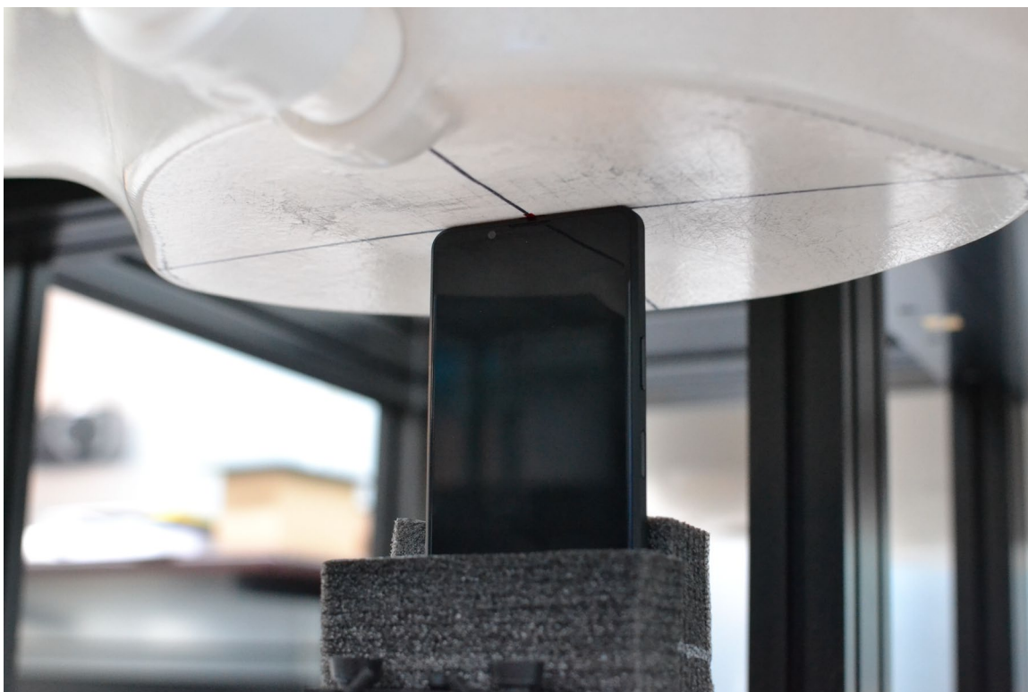
SAR Test Setup Photo 10 – Phablet, Top Edge, 0 mm
