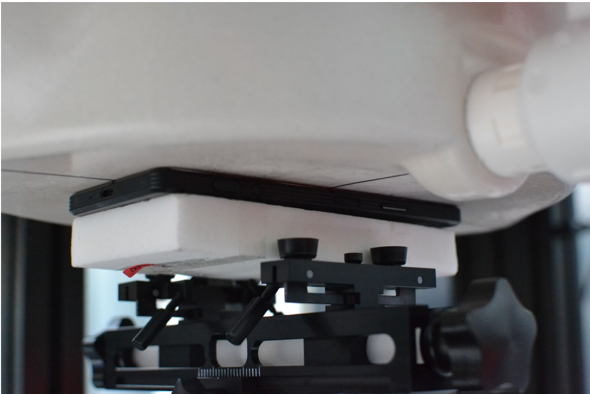
SAR Test Setup Photo 8 – Phablet, Front Side, 0 mm
