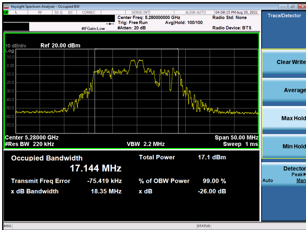
Plot 7-60. 26dB Bandwidth Plot SISO ANT2 (20MHz BW 802.11ax – 26 Tones (UNII Band 2A) – Ch. 56)
