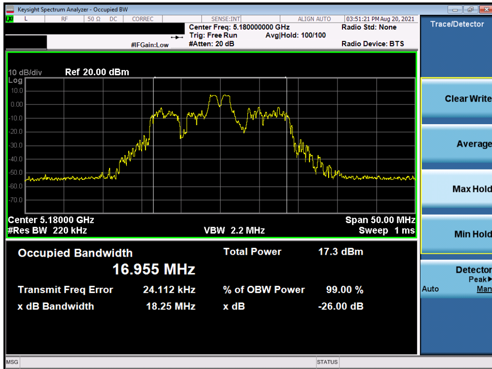
Plot 7-51. 26dB Bandwidth Plot SISO ANT2 (20MHz BW 802.11ax – 26 Tones (UNII Band 1) – Ch. 36)
