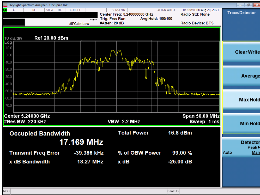
Plot 7-53. 26dB Bandwidth Plot SISO ANT2 (20MHz BW 802.11ax – 26 Tones (UNII Band 1) – Ch. 48)
