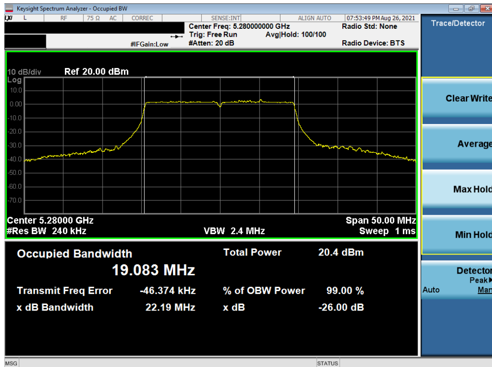
Plot 7-35. 26dB Bandwidth Plot SISO ANT1 (20MHz BW 802.11ax – 242 Tones (UNII Band 2A) – Ch. 56)
