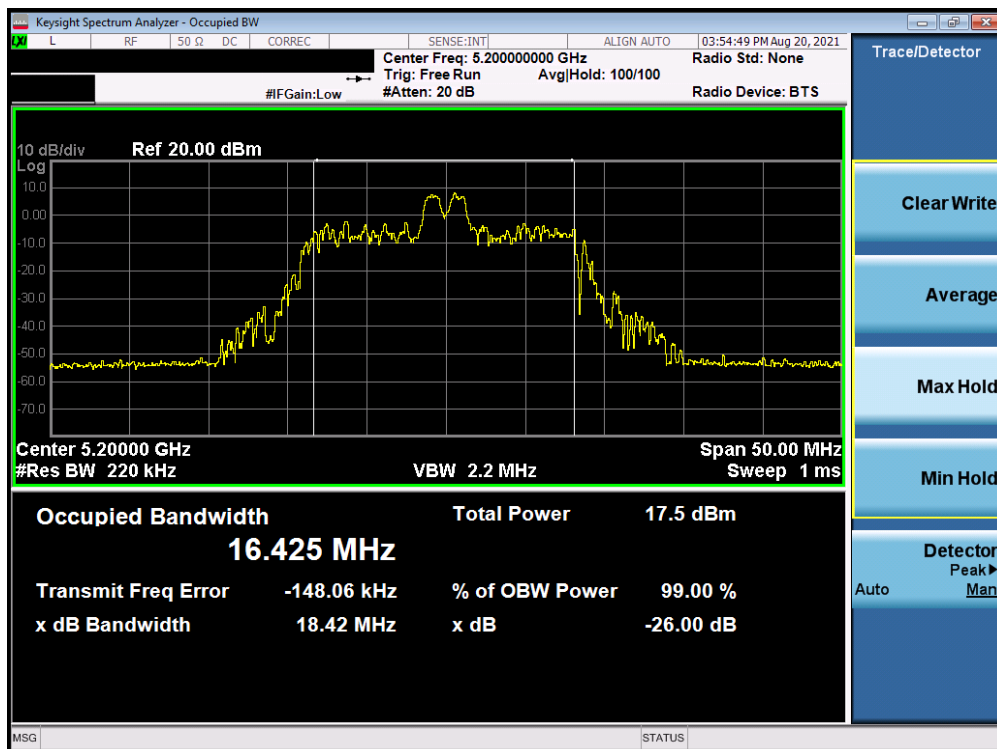
Plot 7-52. 26dB Bandwidth Plot SISO ANT2 (20MHz BW 802.11ax – 26 Tones (UNII Band 1) – Ch. 40)
