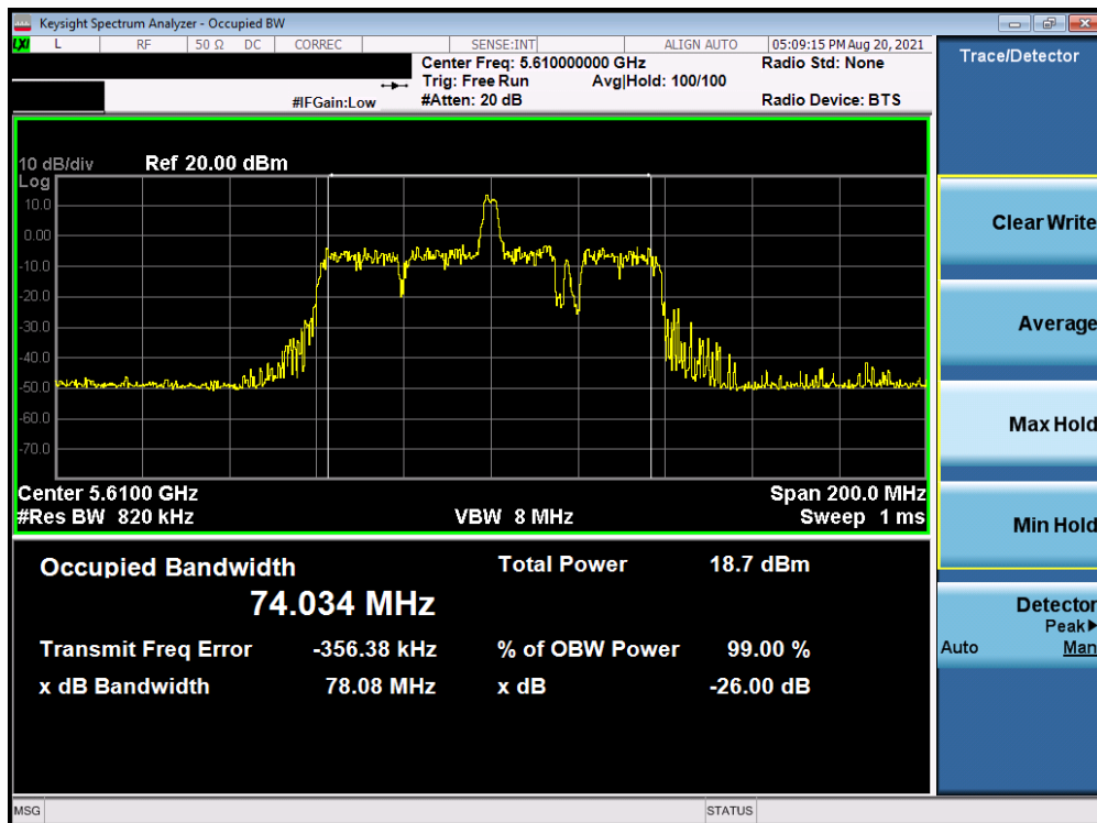
Plot 7-72. 26dB Bandwidth Plot SISO ANT2 (80MHz BW 802.11ax – 26 Tones (UNII Band 2C) – Ch. 122)
