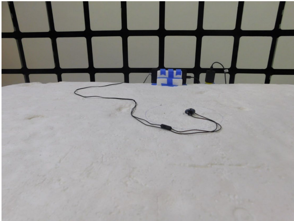
Photo of test setup for Radiated Emissions: 30-1000 MHz Power Supply, WWAN Rx
