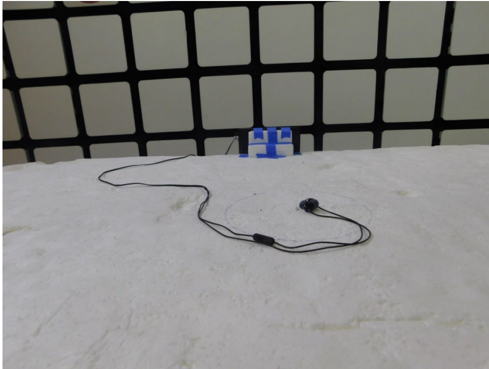
Photo of test setup for Radiated Emissions: >1 GHz Battery
