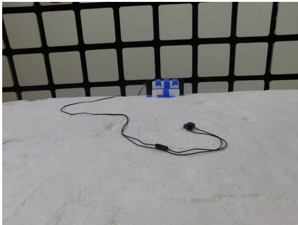
Photo of test setup for Radiated Emissions: 30-1000 MHz Battery
