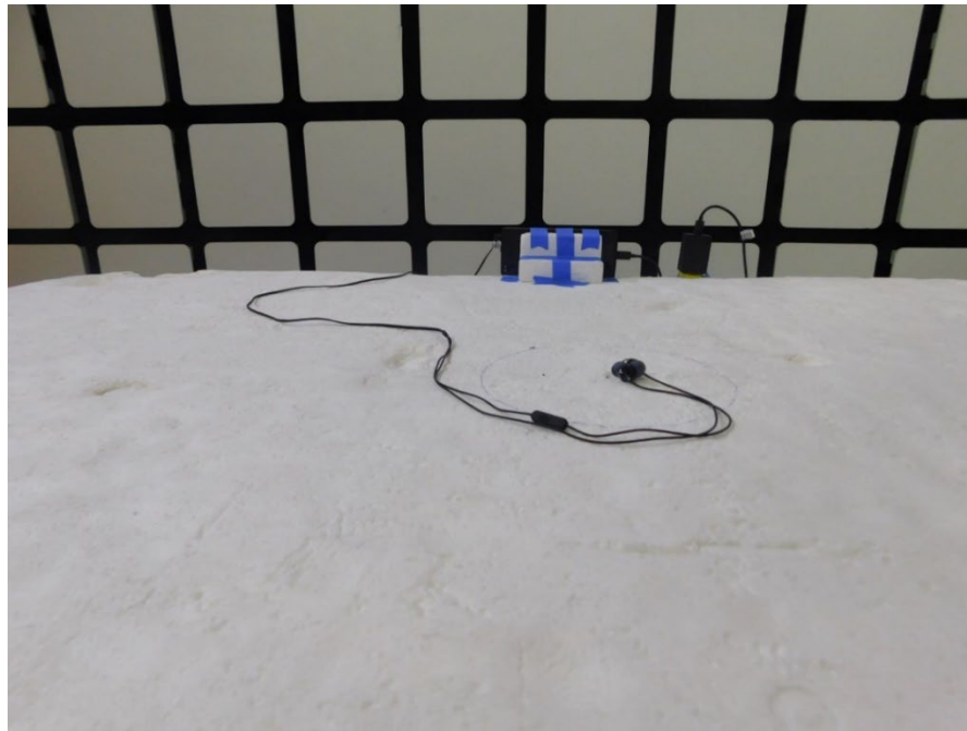
Photo of test setup for Radiated Emissions: >1 GHz Power Supply, WWAN Rx
