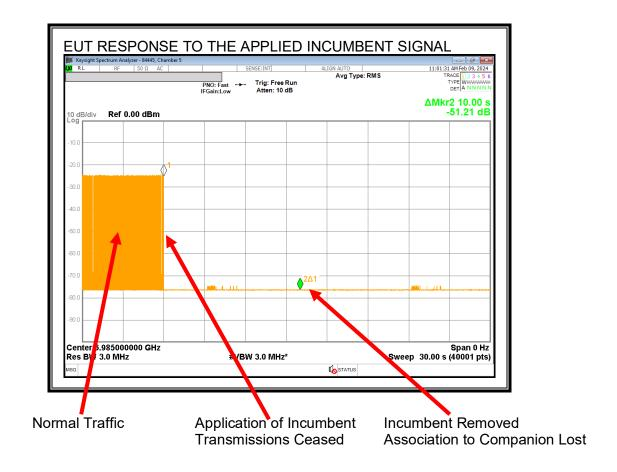
Transmissions cease while the Incumbent AWGN Signal is present and does not resume after it is removed due to the loss of the association to the Companion Device.
