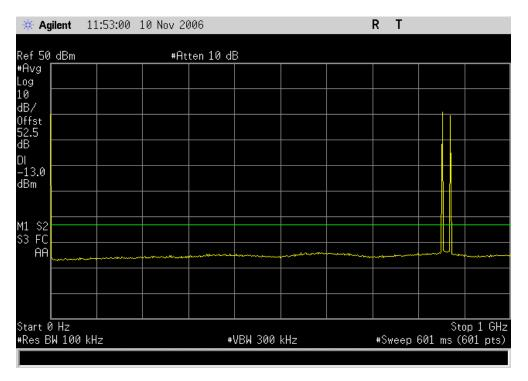
3 Channel Intermods, 995MHz-2.8GHz **Result:** Pass **Value:** <-25 dBm **Limit:** ≤-13 dBm
