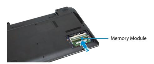
Push the memory module down so that it is completely fixed. If the memory does not fit easily, push the memory module down while pulling the memory module latches outward.
