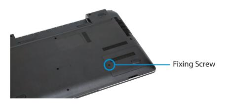
**7** Remove the screws from the memory slot cover to remove it.
