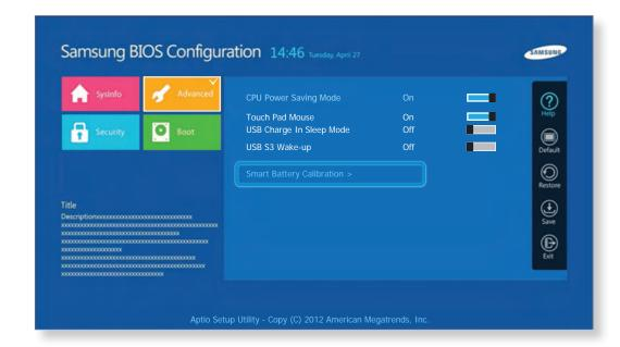
The Battery Calibration function is activated and the battery is forcefully discharged. To stop the operation, press the <**Esc**> button.
