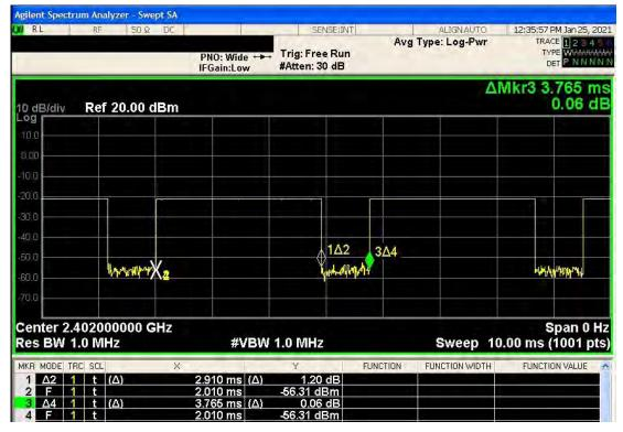
The SAR evaluation of this device selected 1M with the highest average power and the duty cycle is 77.3.
