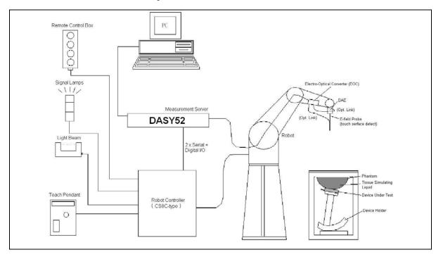
The DASY52 system for performing compliance tests consists of the following items:
