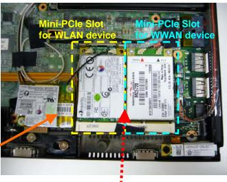
The certification label is stuck on the topside of the applying transmitter device, and
