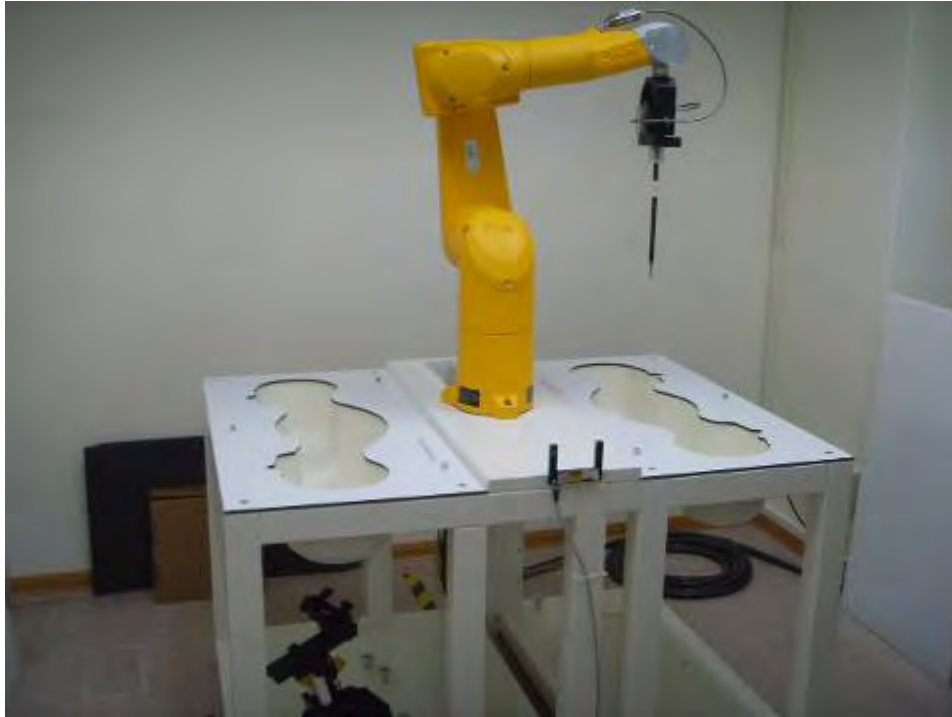
Fig.1 Photograph of the SAR measurement System
