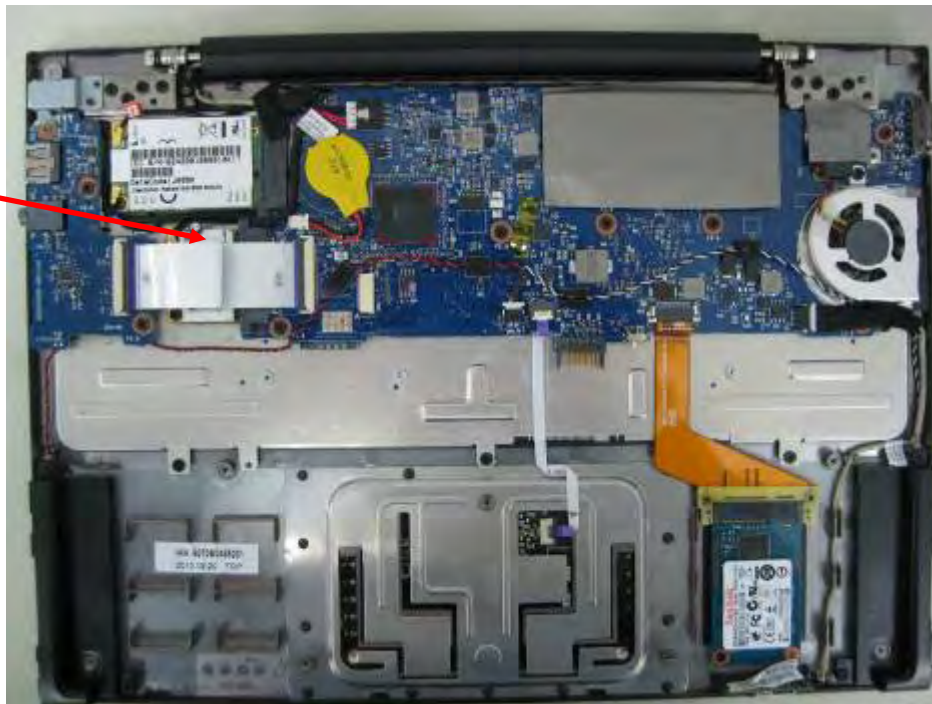
Fig.6 WLAN Module position of EUT
