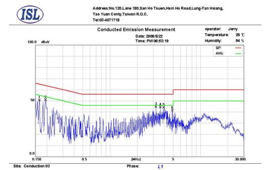
Limit: CISPR22 Class B Conduction(QP)
