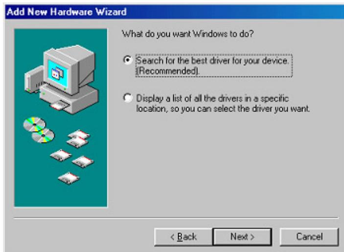
3. Insert the Atheros Software Release CD in the CD-ROM drive. Choose "Specify a location" and browse to the location where the NDIS driver is located. The default folder is **D:\ndis\bin\production\install** (assuming D: is the CD-ROM drive).
