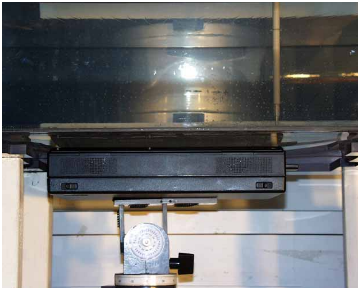
< Bottom of the host PC faced toward the phantom – 17 mm (Card-to-Bottom) >
