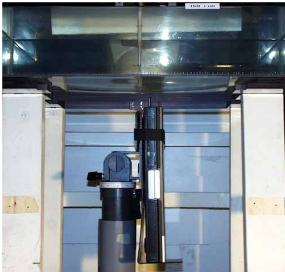
< Edge of the card pointed toward the phantom, 10 mm separation distance, Prescan >
