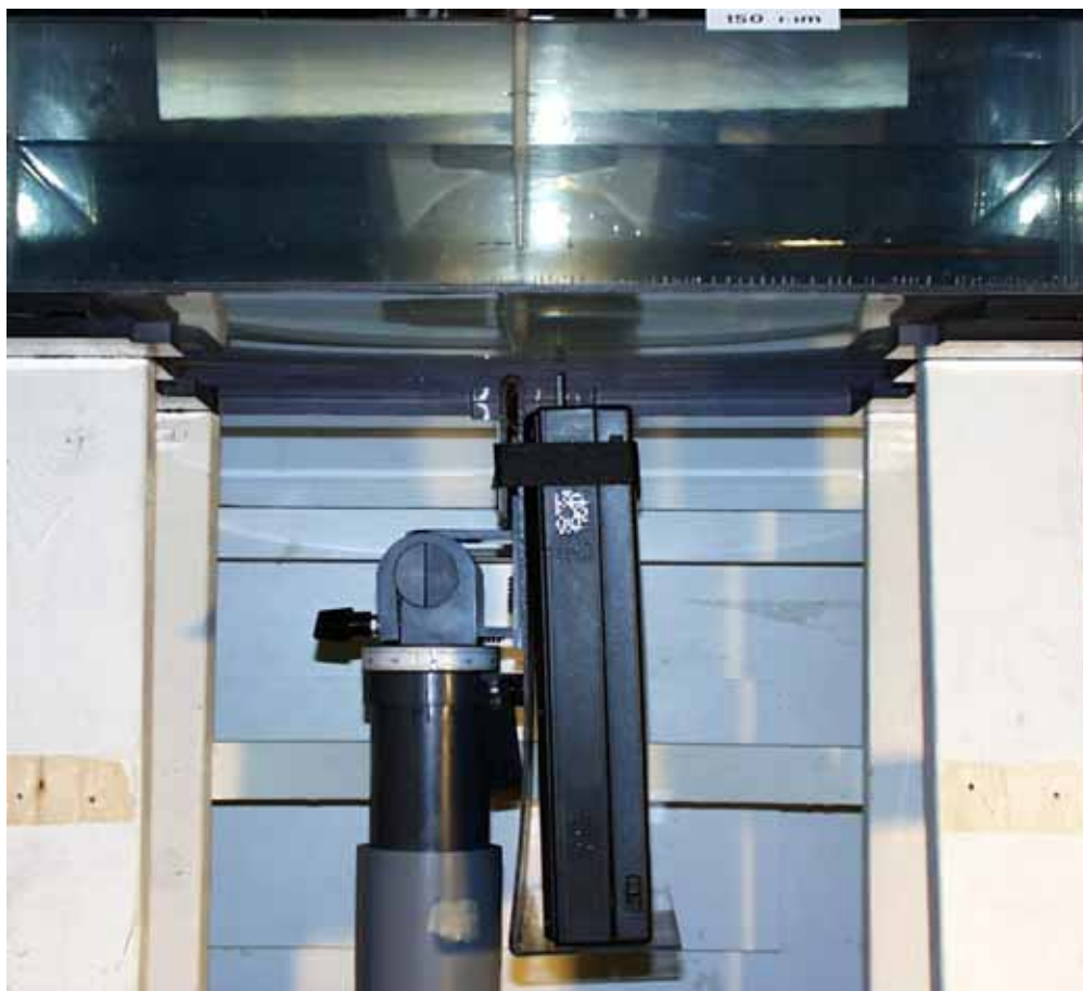
< Edge of the card pointed toward the phantom, 10 mm separation distance, Prescan >
