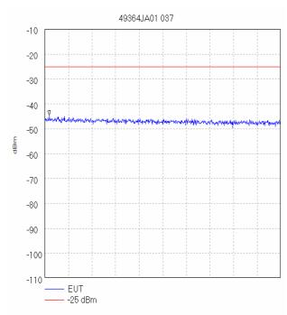
Start 26.5 GHz; Stop 27.0 GHz Ref -10 dBm; Ref Offset 43.0 dB; 10 dB/div RBW 1.0 MHz; VBW 1.0 MHz; Att 0 dB; Swp 50.0 mS Peak 26.509167 GHz, -44.5 dBm
