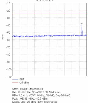
Peak 1.933333 GHz, -39.5 dBm Display Line: -25 dBm; ; Limit Test Passed Tested by jxh 30/08/2007 13:43:20
