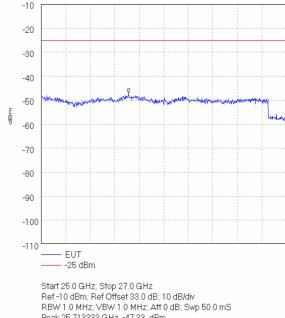
Peak 25.713333 GHz, -47.33 dBm Display Line: -25 dBm; ; Limit Test Passed Tested by jxh 30/08/2007 13:50:36
