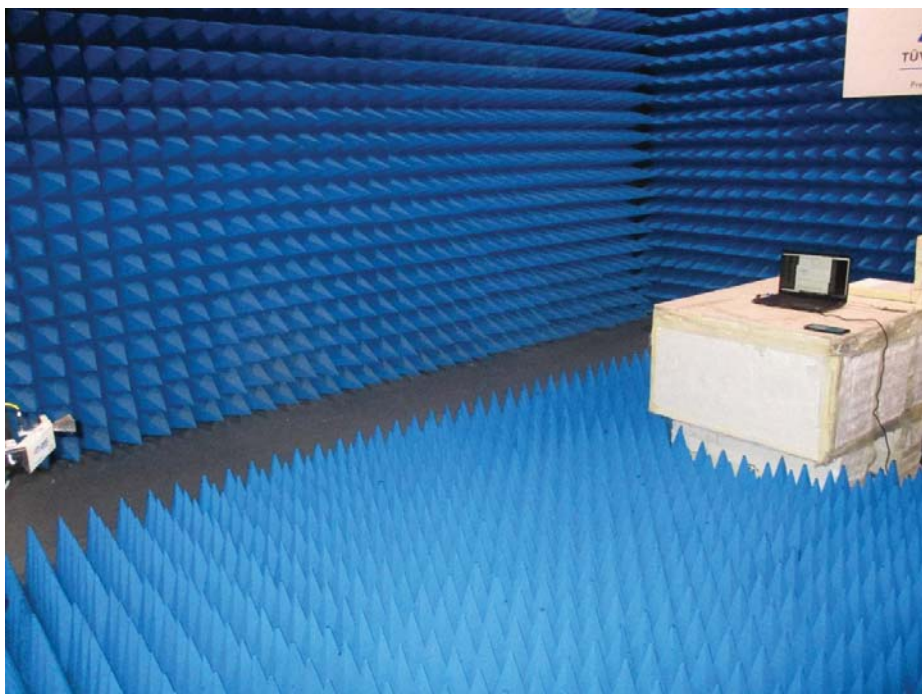
Photo 3: Photograph radiated emissions 18 – 26.5 GHz
