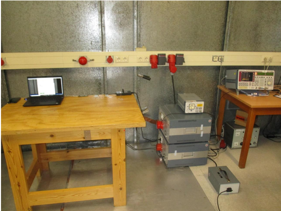
Photo 5: Photograph conducted emissions 0.15-30 MHz
