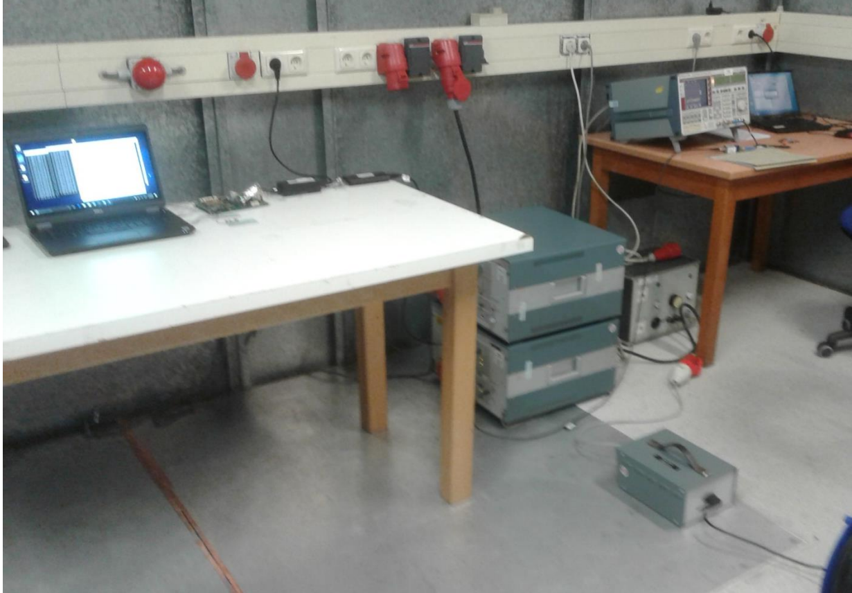
Photo 5: Photograph conducted emissions 0.15-30 MHz
