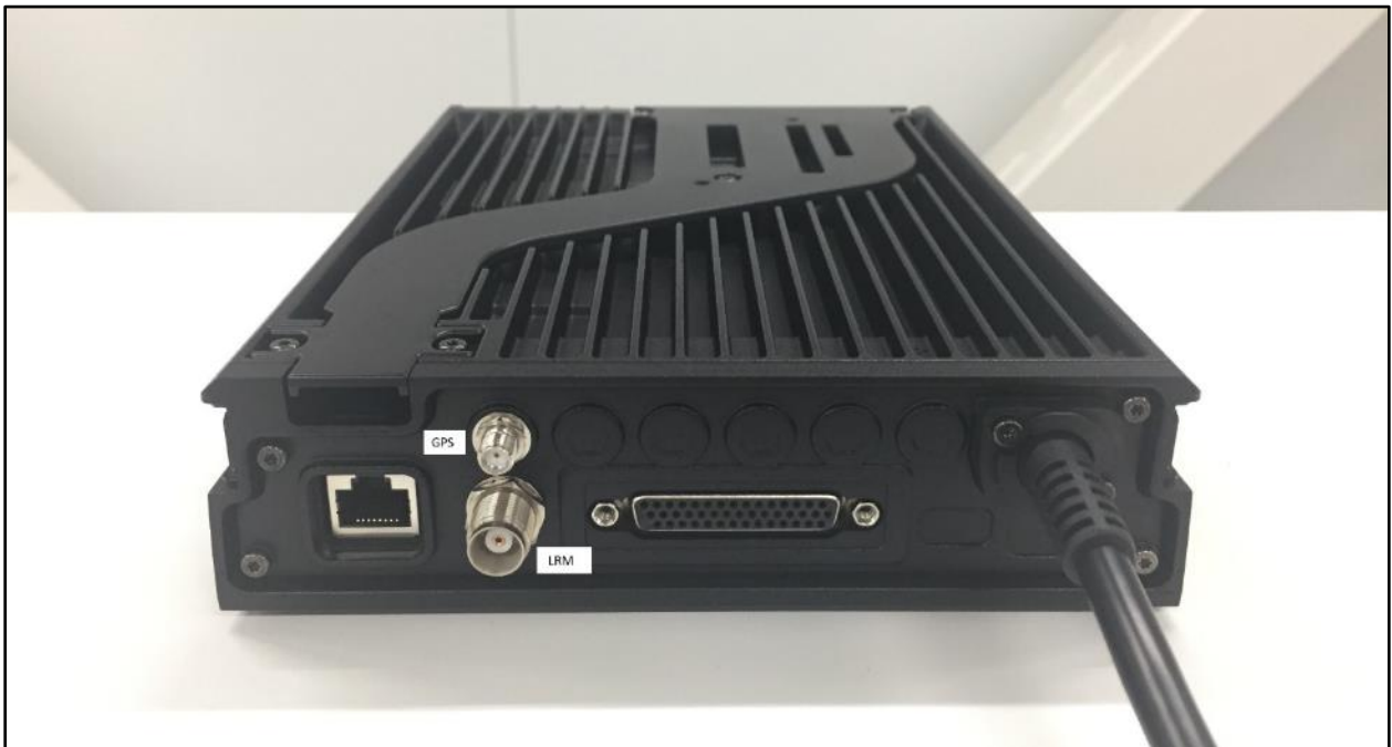
VCH Rear with Antenna Connectors
