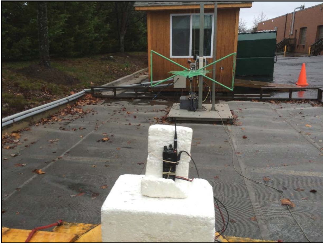
Photograph 3: Radiated Emissions Testing – Front View <1 GHz
