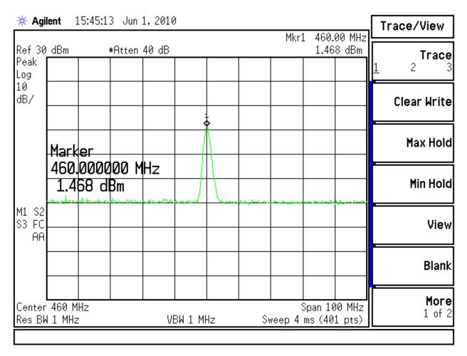
Using the attenuation factor at 460 MHz frequency:
