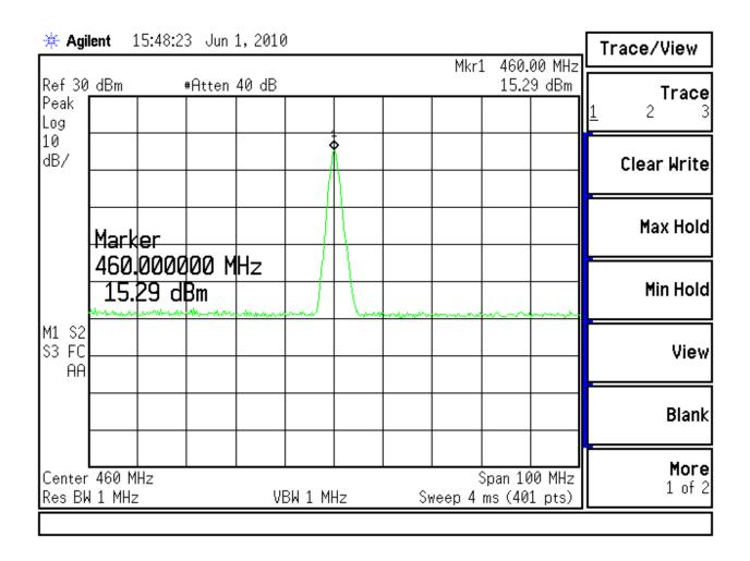
Using the attenuation factor at 460 MHz frequency:
