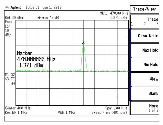
Using the attenuation factor at 470 MHz frequency:
