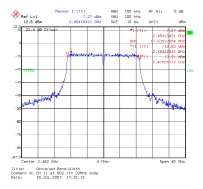
DAC1: 99% Occupied Bandwidth @ draft 802.11n 40MHz mode channel 3
