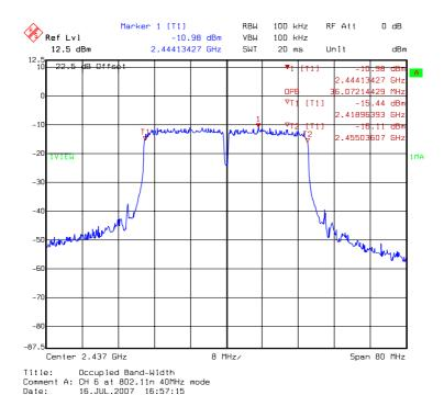
DAC1: 99% Occupied Bandwidth @ draft 802.11n 40MHz mode channel 9
