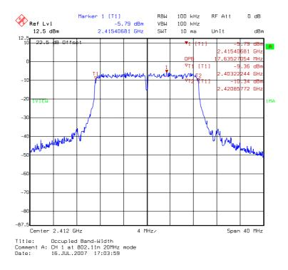
DAC1: 99% Occupied Bandwidth @ draft 802.11n 20MHz mode channel 6
