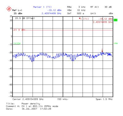
DAC1: Power Spectral Density @ draft 802.11n 20MHz mode channel 6
