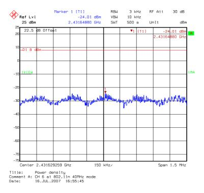
DAC1: Power Spectral Density @ draft 802.11n 40MHz mode channel 9
