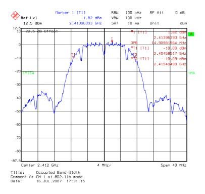
DAC1: 99% Occupied Bandwidth @ 802.11b mode channel 6
