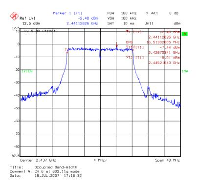
DAC1: 99% Occupied Bandwidth @ 802.11g mode channel 11
