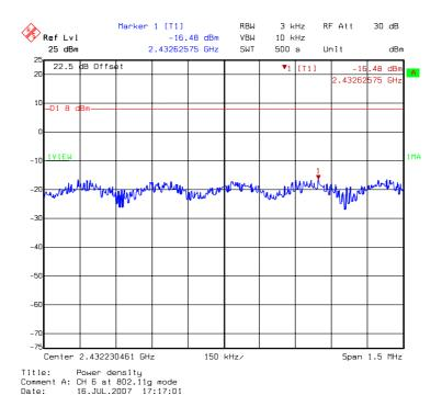
DAC1: Power Spectral Density @ 802.11g mode channel 11
