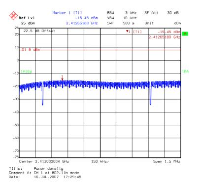
**DAC1:** Power Spectral Density @ 802.11b mode channel 6
