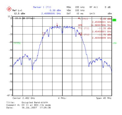
DAC1: 99% Occupied Bandwidth @ 802.11g mode channel 1
