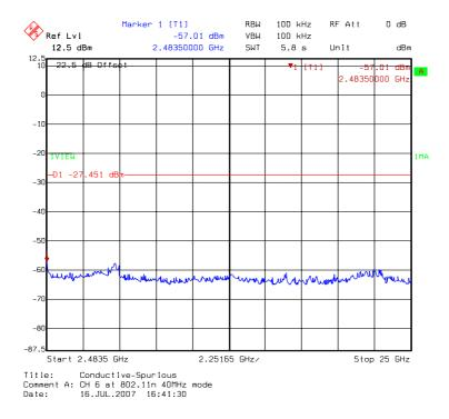
DAC0: conducted spurious @ draft 802.11n 40MHz mode channel 9 (1 of 3)
