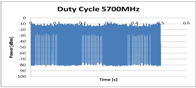
Note: The Duty Cycle of 49.1% was calculated from the raw data used to generate this plot. A longer sweept time will result in incorrect calculation of the duty cycle as no more than 25k trace points are available.
