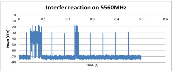
Note: The 0.24ms accumulated transmit time was calculated from the raw data used to generate this plot. A longer sweept time will result in incorrect calculation of the duty cycle as no more than 25k trace points are available.
