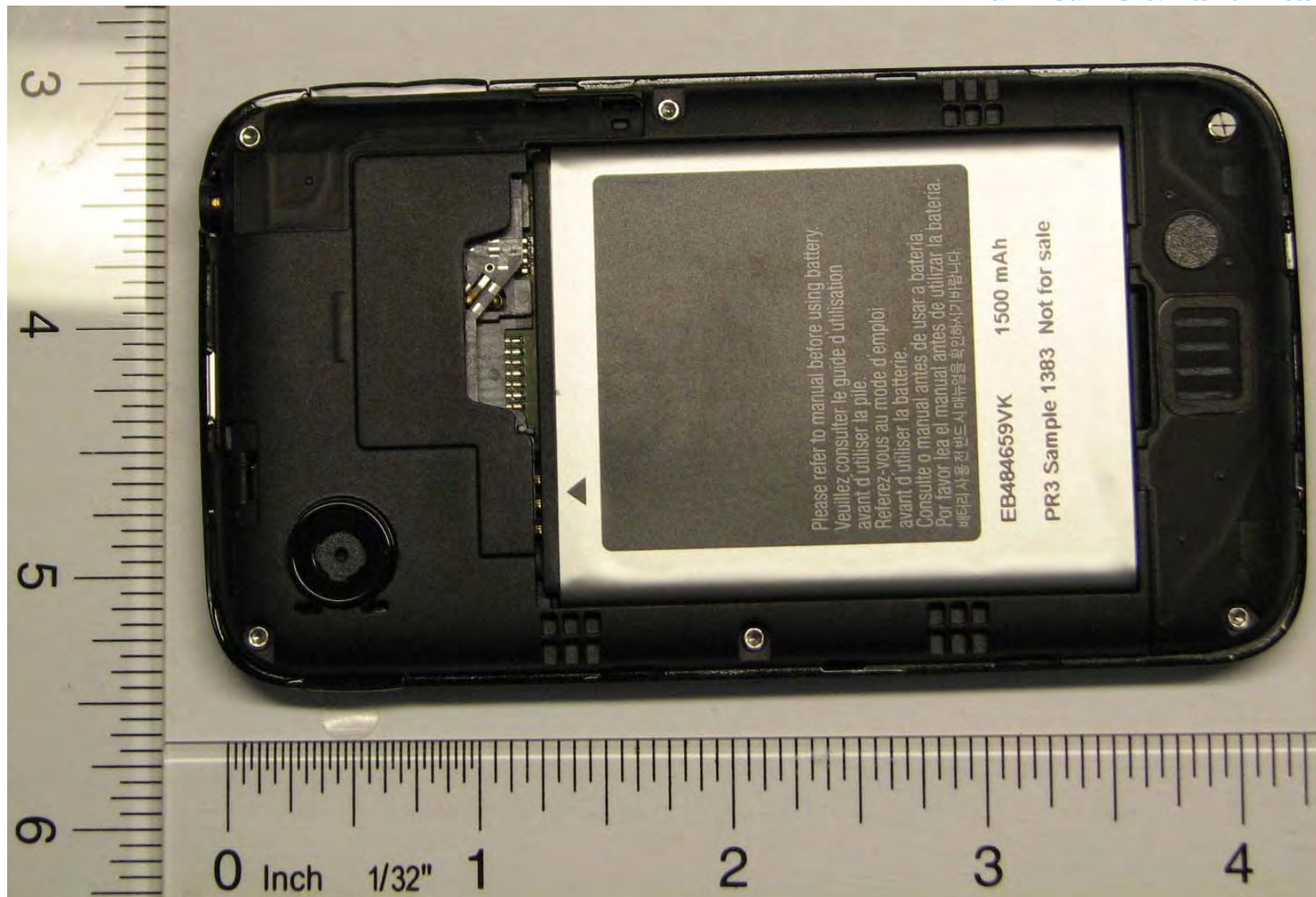
Figure 2: BT210/BT230/BT510 with back cover removed
