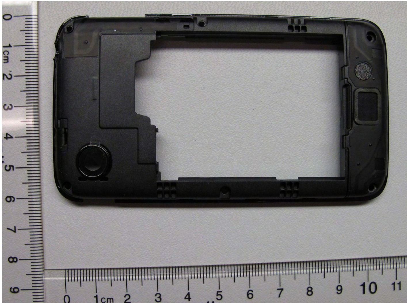
Figure 4: BT and GPS antenna back side
