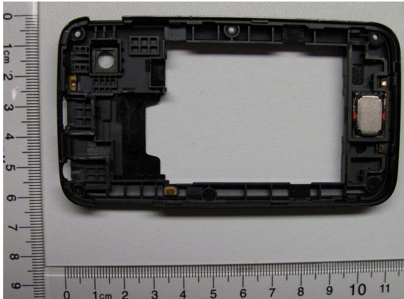
Figure 5: Cellular antenna front side
