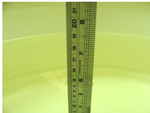
Fig 6.2 Photo of Liquid Height for Body SAR
