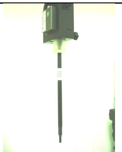
Fig 5.2 Photo of ET3DV6/ET3DV6R
