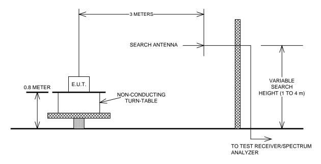
The spectrum was searched up to the 10th harmonic of the fundamental frequency of operation. Note:
