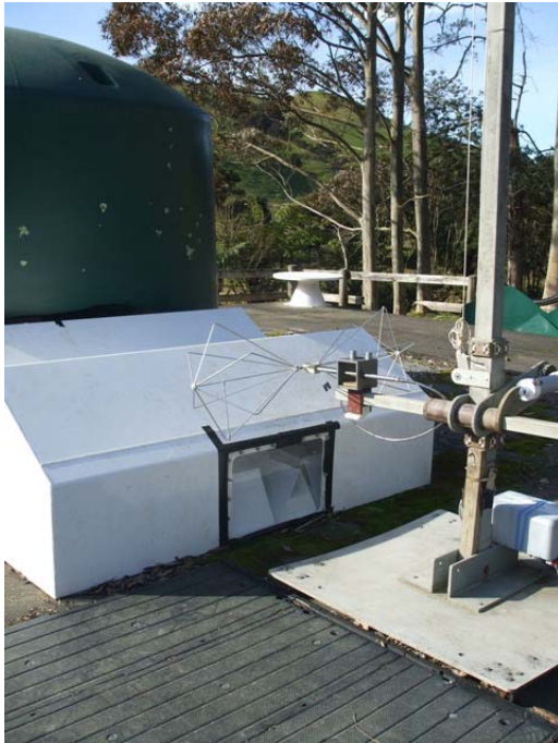
Test set up using a biconical antenna between 30 - 300 MHz
