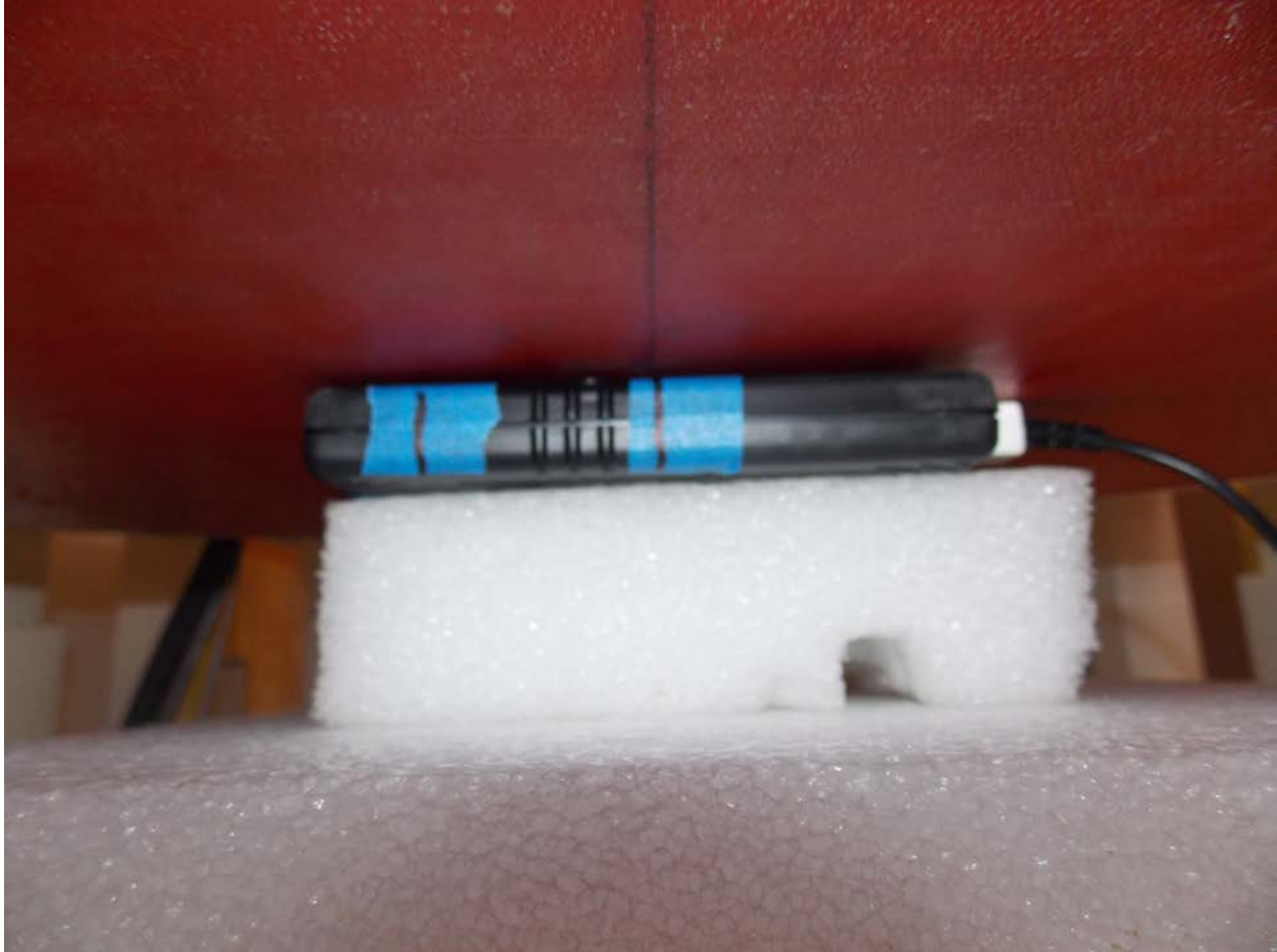
Test Position Eli Flat Front Facing Phantom 0 mm Gap
