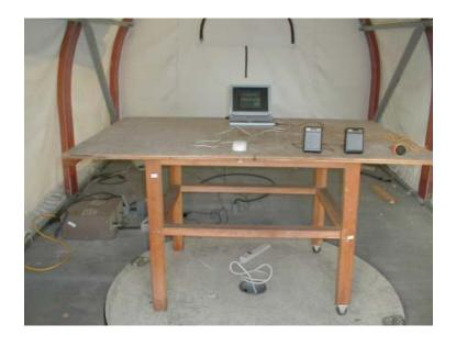
**Conducted Emission Test Setup – Rear View**
