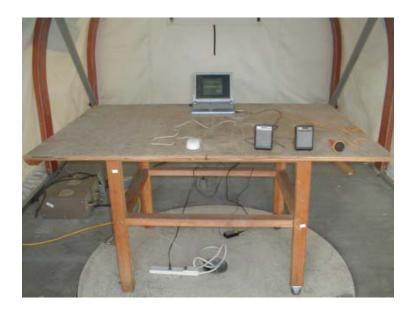
$Radiated\ Emission\ Test\ Setup-Rear\ View$
