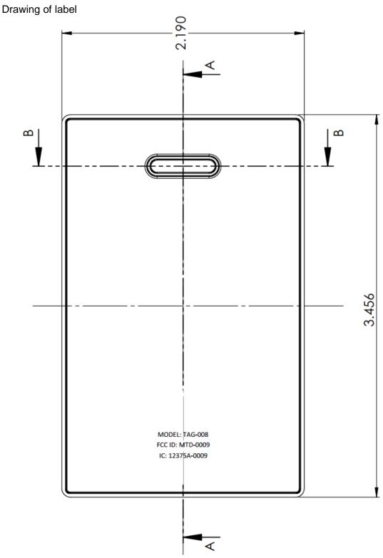
The Label will be etched onto the EUT Dimensions are in inches
