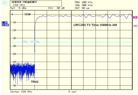
The results of testing the URC-200 rising RF envelope during the "Transmit Transient" condition is plotted below in FM 158 MHz.
