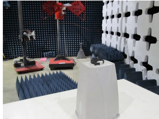
Radiated emissions test set up above 1GHz.
