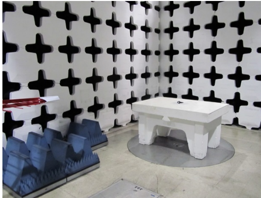
Radiated emissions test set up below 1GHz.
