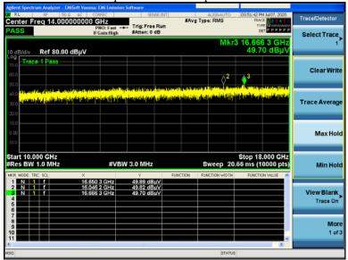
Transmitter Radiated Spurious Emissions peak vertical 10GHz – 18GHz (BLE 2402MHz)
