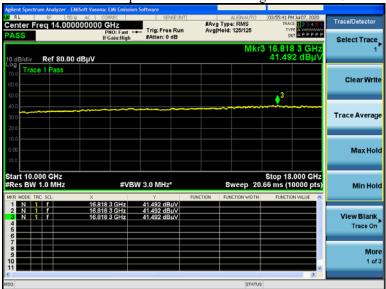
Transmitter Radiated Spurious Emissions average vertical 10GHz – 18GHz (BLE 2442MHz)
