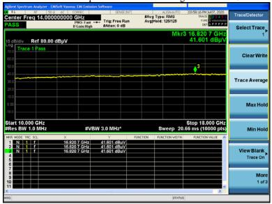
Transmitter Radiated Spurious Emissions average vertical 10GHz – 18GHz (BLE 2480MHz)
