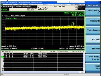
Tx Spurious Emissions 10GHz-18GHz. 2412MHz peak vertical
