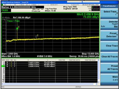
Tx Spurious Emissions 1GHz-10GHz. 2442MHz peak vertical
