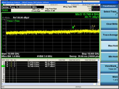
Tx Spurious Emissions 10GHz-18GHz. 2442MHz peak vertical
