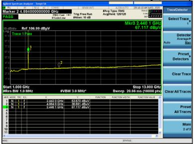
Tx Spurious Emissions 1GHz-10GHz. 2442MHz average (vertical polarity)
