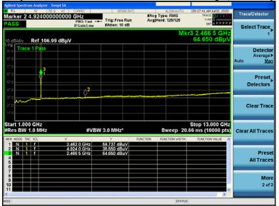
Tx Spurious Emissions 1GHz-10GHz. 2462MHz average (vertical polarity)
