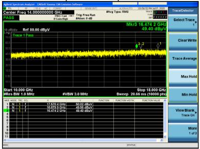
Transmitter Radiated Spurious Emissions peak vertical 10GHz – 18GHz (BLE 2480MHz)
