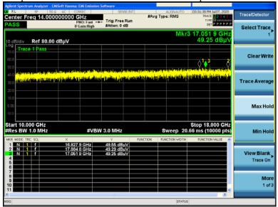
Tx Spurious Emissions 10GHz-18GHz. 2462MHz peak vertical
