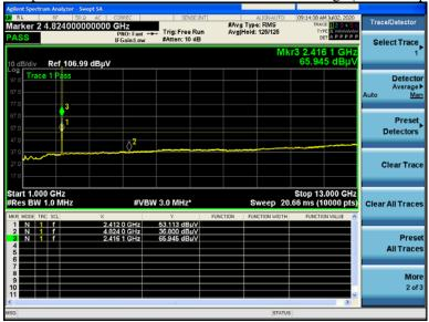
Tx Spurious Emissions 1GHz-10GHz. 2412MHz average (vertical polarity)
