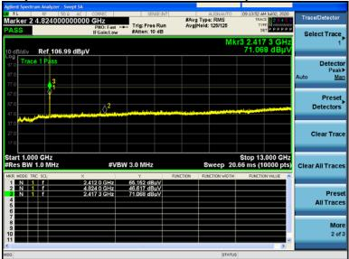
Tx Spurious Emissions 1GHz-10GHz. 2412MHz peak vertical
