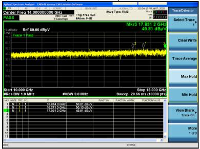
Transmitter Radiated Spurious Emissions peak vertical 10GHz – 18GHz (BLE 2442MHz)
