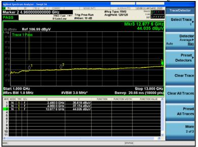
Tx Spurious Emissions 1GHz-10GHz. BLE 2480MHz average vertical
