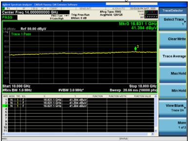
Transmitter Radiated Spurious Emissions average vertical 10GHz – 18GHz (BLE 2402MHz)
