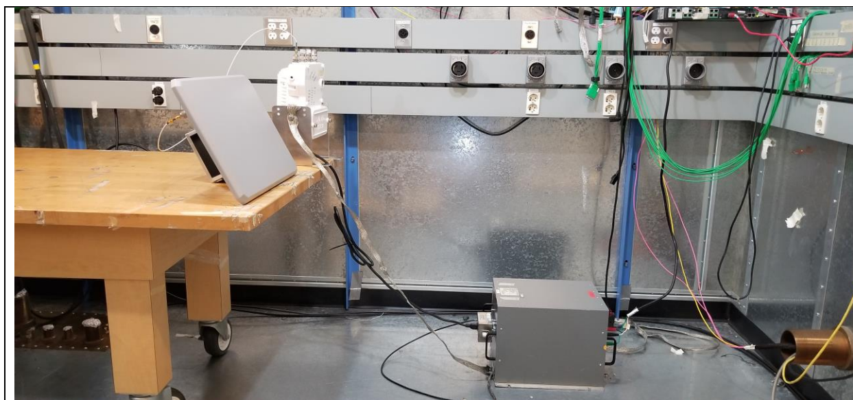
Title: Conducted Emissions 150KHz-30MHz – Test Setup
