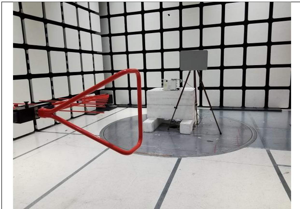
Title: Radiated Spurious Emissions 30MHz-1GHz – Test Setup
