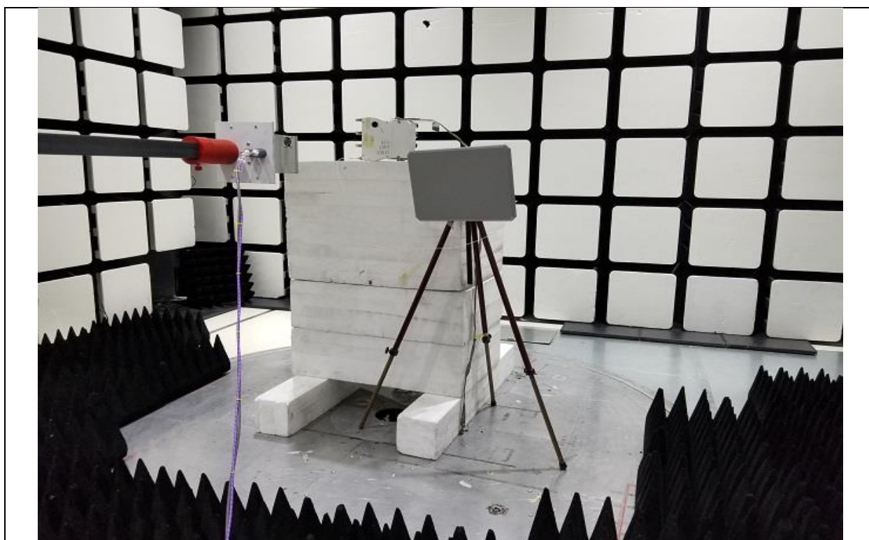
Title: Radiated Spurious Emissions 18GHz-40GHz – Test Setup
