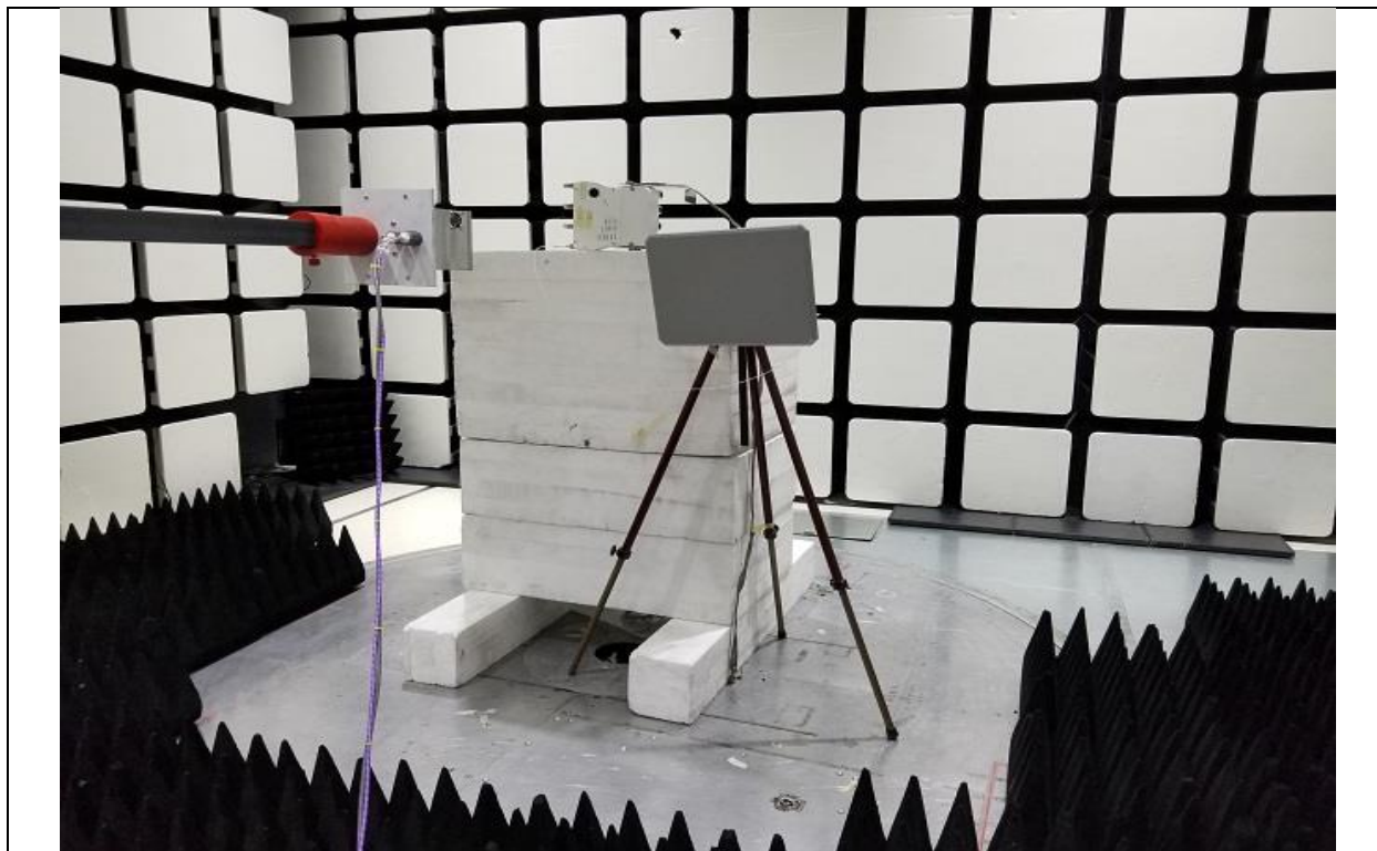
Title: Radiated Spurious Emissions 18GHz-40GHz – Test Setup
