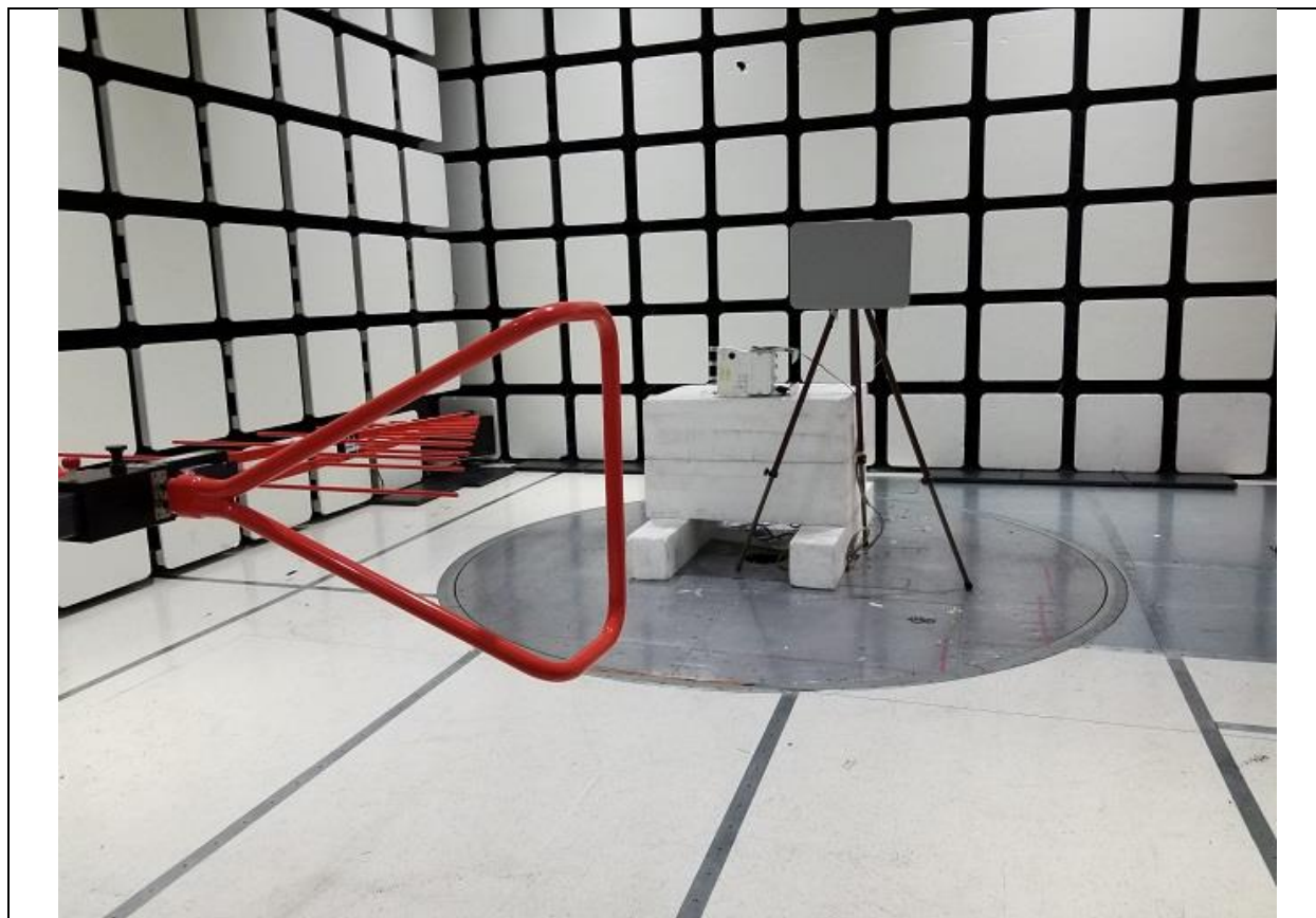
Title: Radiated Spurious Emissions 30MHz-1GHz – Test Setup
