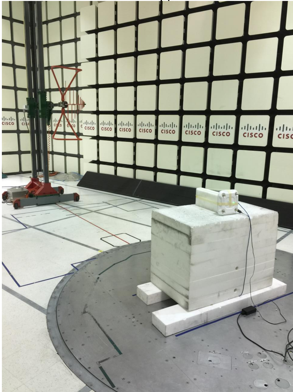
AIR-CAP3702E-B-K9 Radiated Test setup photo 30MHz to 1GHz
