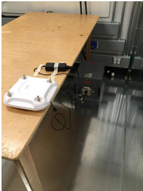
AIR-CAP3702E-B-K9 AC Conducted Emissions setup photo
