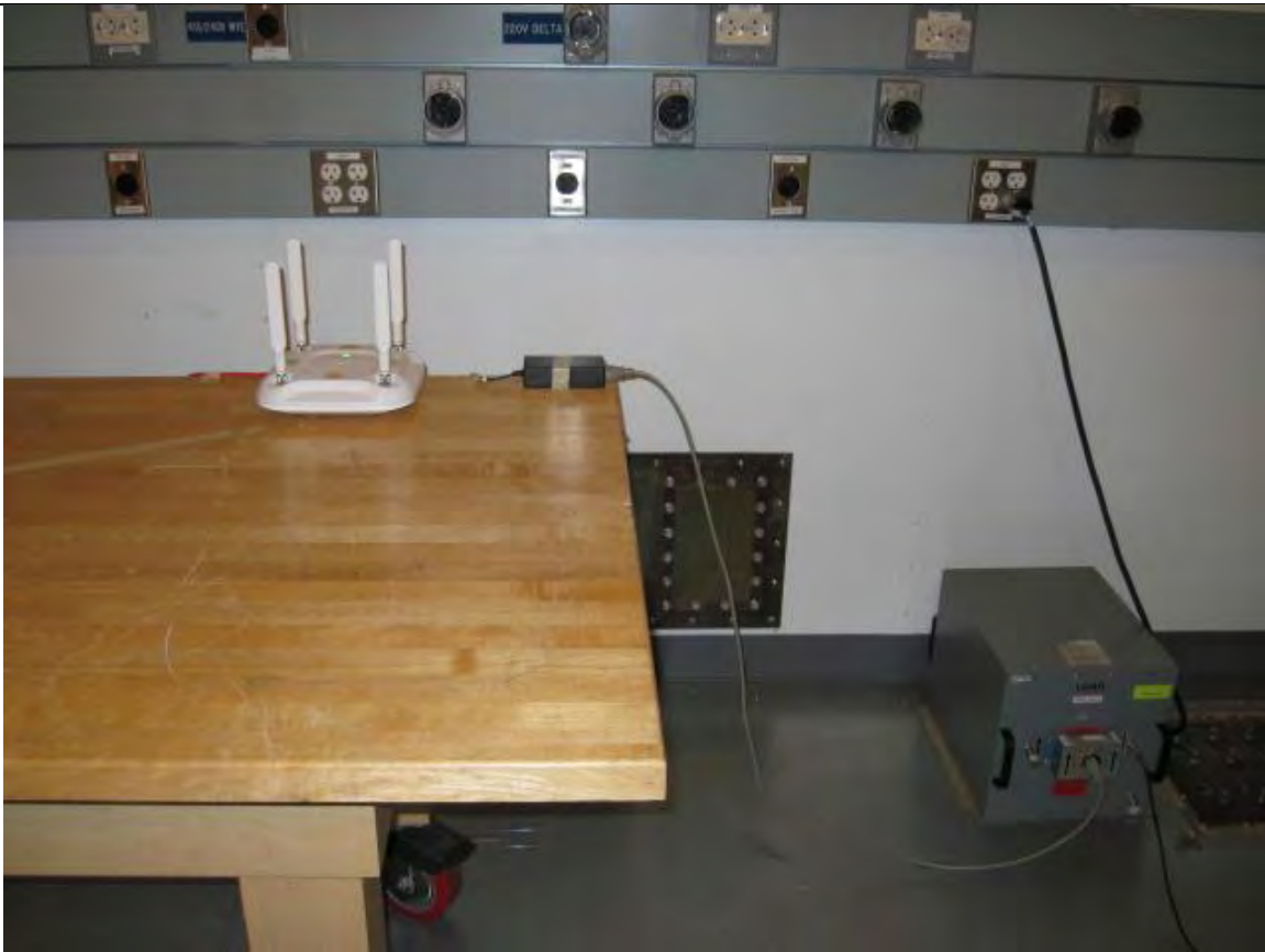
Title: Power Line Conducted Emissions Test Setup
