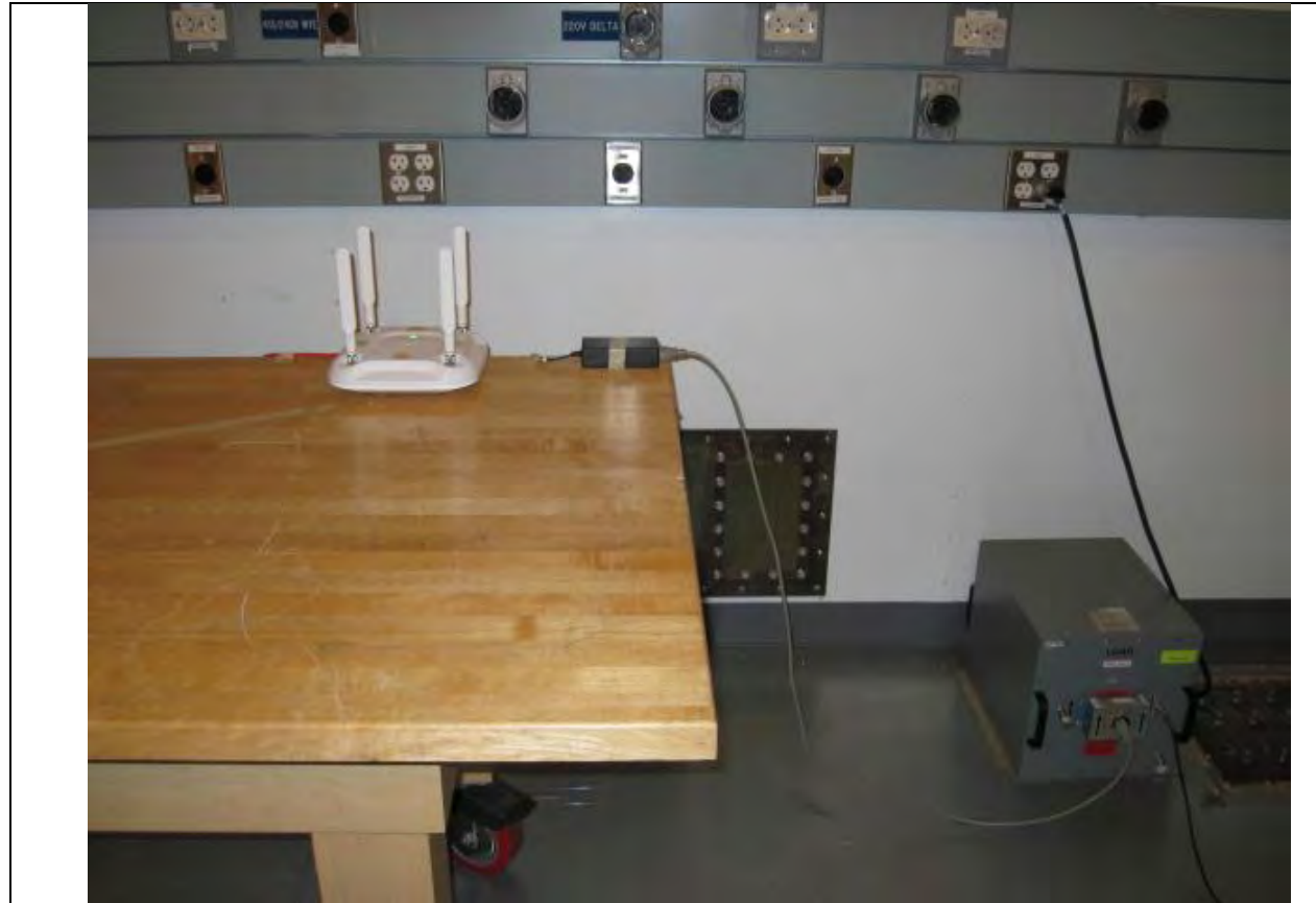
Title: Power Line Conducted Emissions Test Setup
