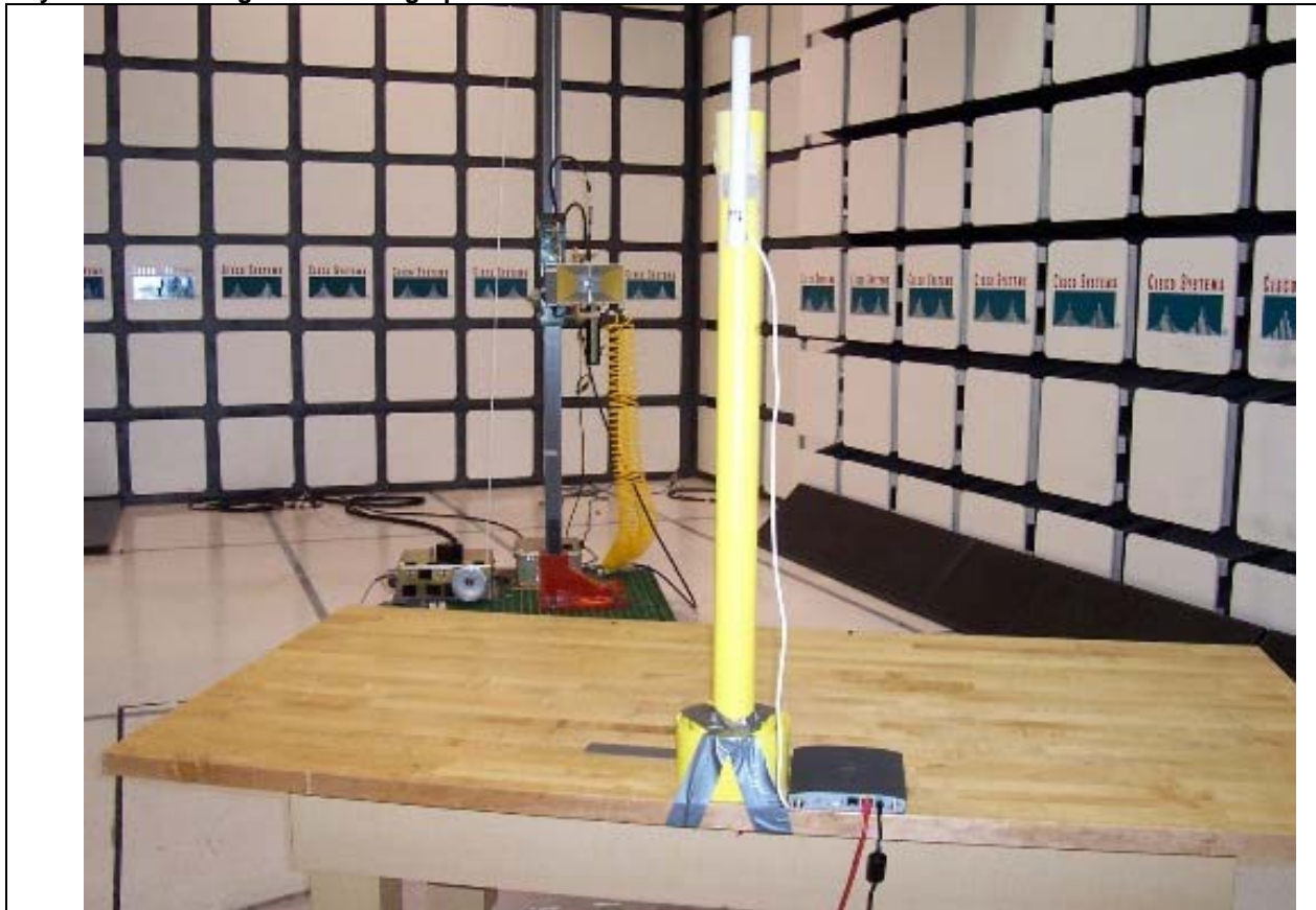
Title: 2.4GHz 5.2dBi Omnidirectional Antenna
