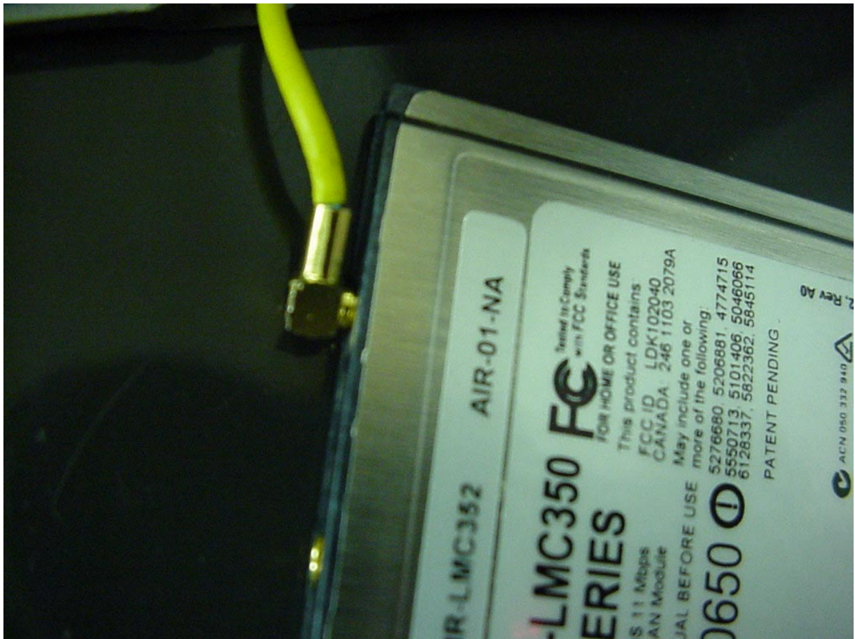
PHOTOGRAPH 12: ANTENNA CONNECTION TO THE WLAN CARD (ITRONIX IX250)
