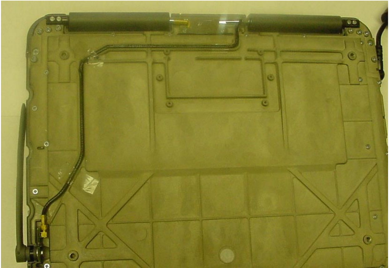
PHOTOGRAPH 15: INSIDE TOP BEZEL SHOWING LOCATION OF CABLING (ITRONIX IX550)
