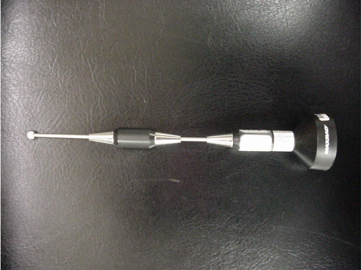
PHOTOGRAPH 9: 5 DBI ANTENNA (ITRNOX IX250)
