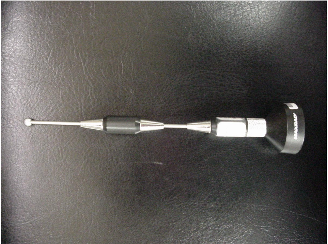
PHOTOGRAPH 17: 5 DBI ANTENNA (ITRONIX IX550)
