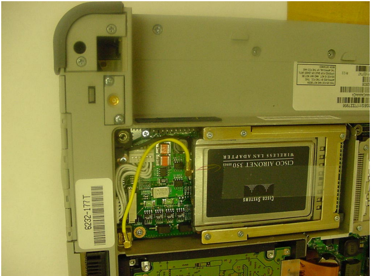
PHOTOGRAPH 14: INSIDE BOTTOM OF CASE SHOWING CARD (ITRONIX IX550)
