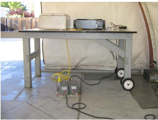
Please note that there is a 2m x 2m Vertical Reference Plane outside the tent @ 40cm spacing from the Master. The measurement LISN is at right, 40cm off the VRP, and the Aux LISN is front and center.
