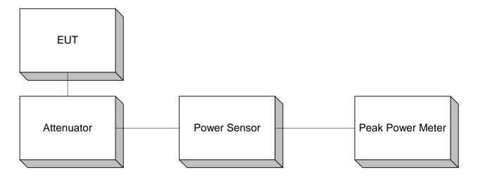
Minimum 6 dB Bandwidth Peak Power Spectral Density Spurious Emissions (conducted)
