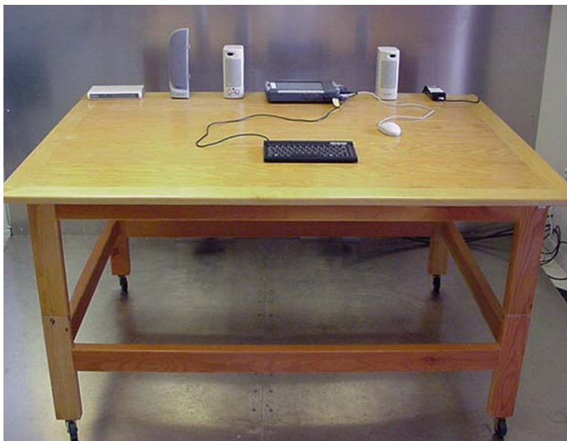
Photograph G-2 - AC Powerline Conducted Emission Configuration
